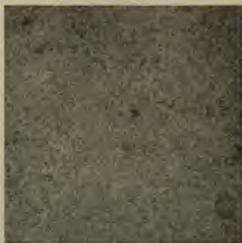
FIG. 16.—Microphotograph of Same Metal, After Repeated Heating at About 1500° F. ( \times 100 ).
